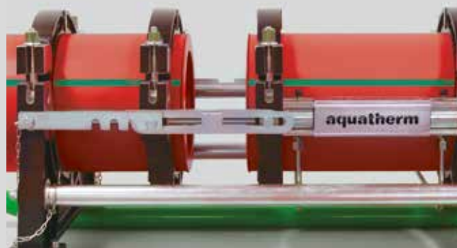
Divide the machine slide, remove heating element
