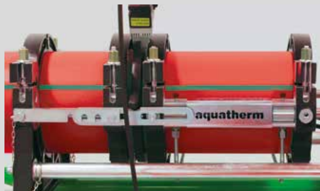
Positioning of heating element
