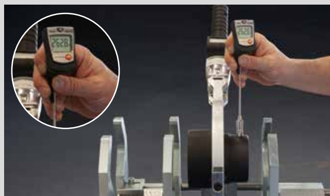
Temperature control aquatherm welding machine
