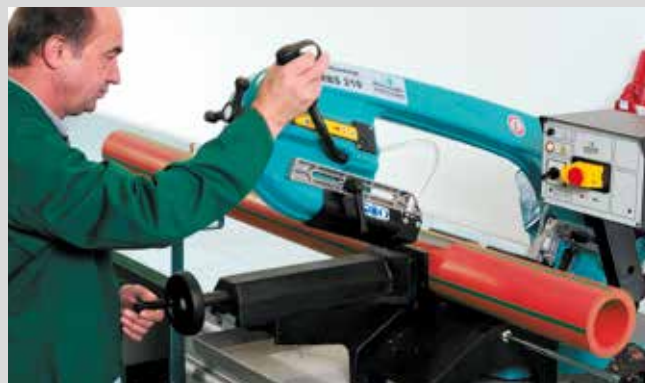
Before welding, pipes are cut into the required lengths
