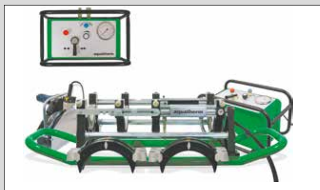
Check performance of the welding machine and heat it up
