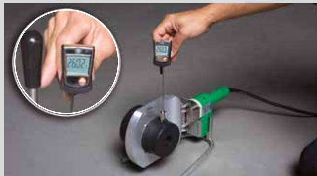
Temperature control aquatherm welding device (1400 W)
